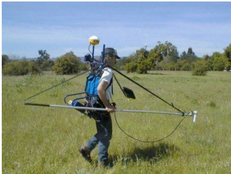
Fig. 1 A Cesium Magnetometer with GPS 31
